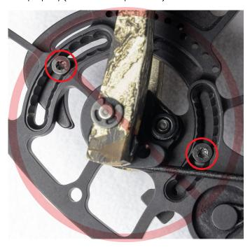
Cable transition from module to cam hub has a gap.
