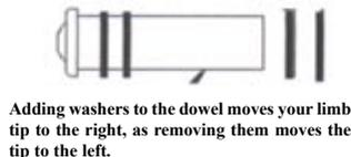
B: remove washers from the sight window side of the dowel. Limit your adjustments to one washer at a time. You can store any unused washers between the riser and alignment cap because
