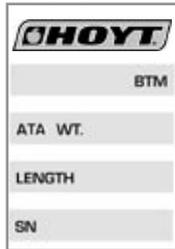
The weight marked on the limb is measured at a 28" standard A.T.A. (Archery Trade Association) draw length. A.T.A. draw length is measured at 26 1/4" to the throat of the bow grip plus 1 3/4". This produces an industry standard by which recurve bows are measured.
