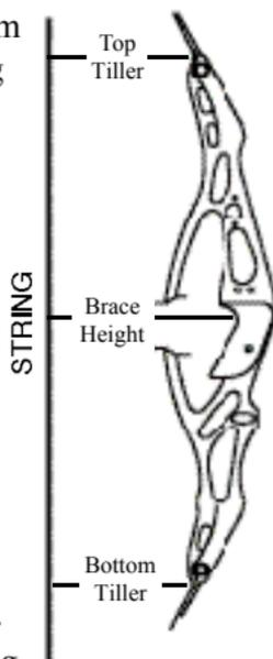
the bottom weight/tiller adjustment bolts in equal but opposite directions. **NOTE: A tiller adjustment will move the nocking point position.**
